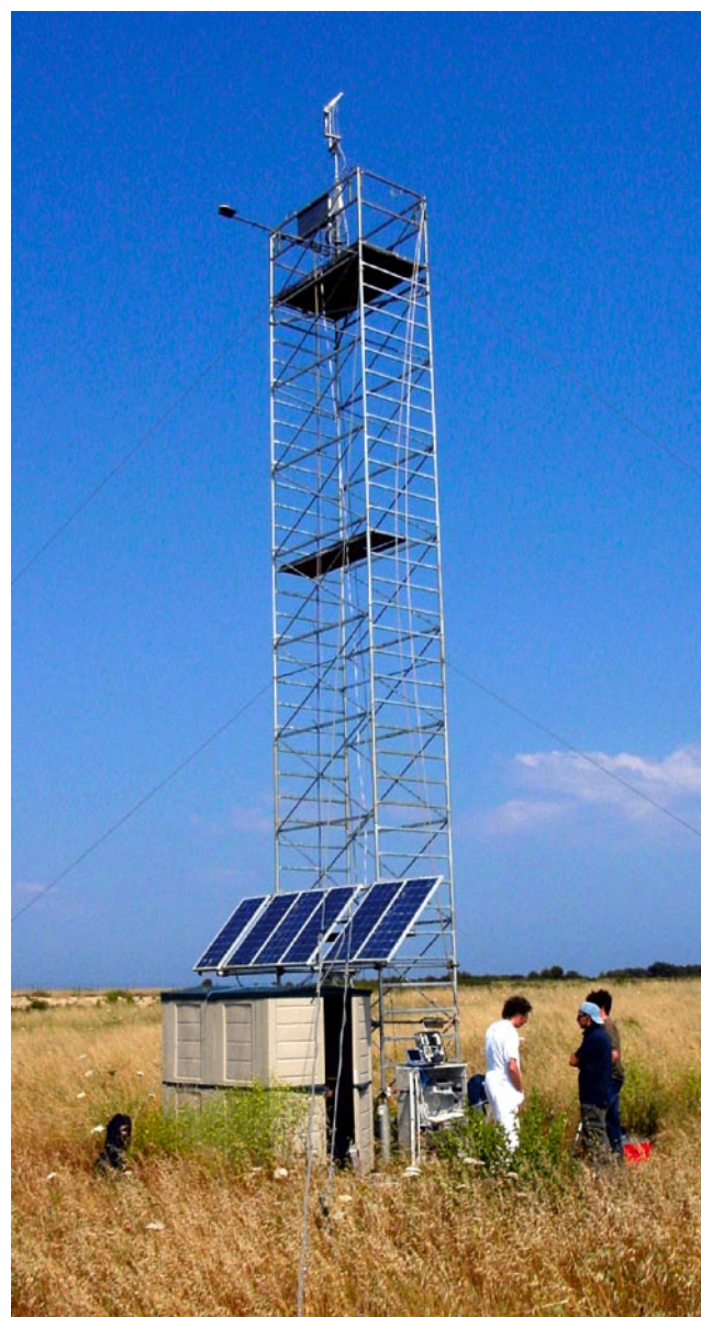
Figure 1 – The eddy covariance tower installed on Pianosa Island
